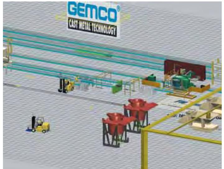
Horizontal moulding line with two induction furnaces
