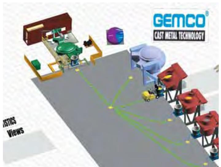
Possible set-up of four induction furnaces, one holder, and one pouring furnace
